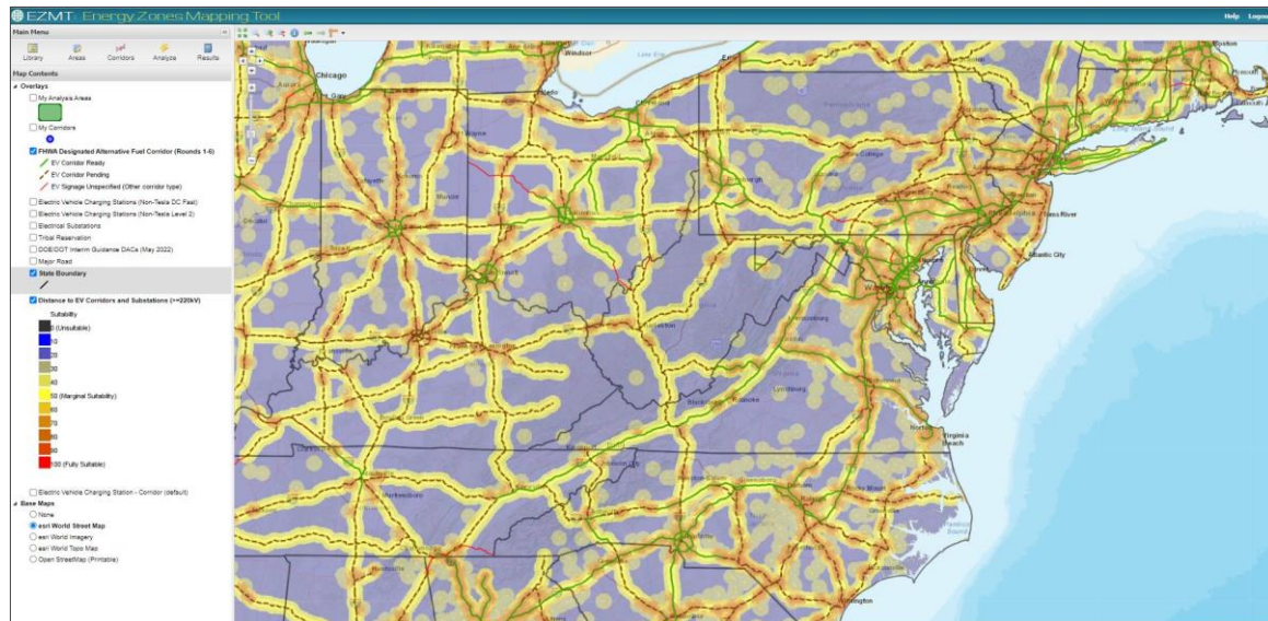
Example EZMT model result showing areas close to Round 6 EV corridors and substations of 220kV and greater
